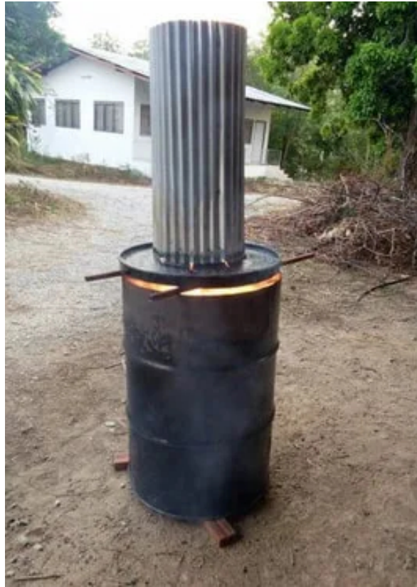
Top-Lit Updraft (TLUD) gasifier for smokeless pyrolytic combustion.
